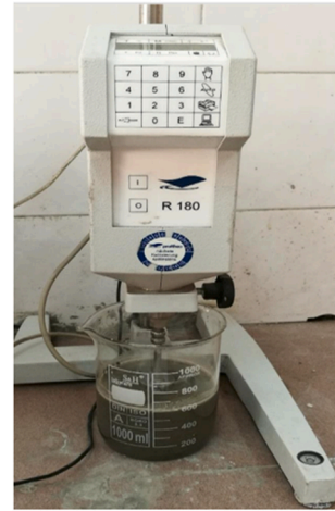
Fig. 3. Rheological properties of jet grout column: (a) Shear stress versus shear rate relationship; (b) Coaxial rotating cylinder Rheometer.
