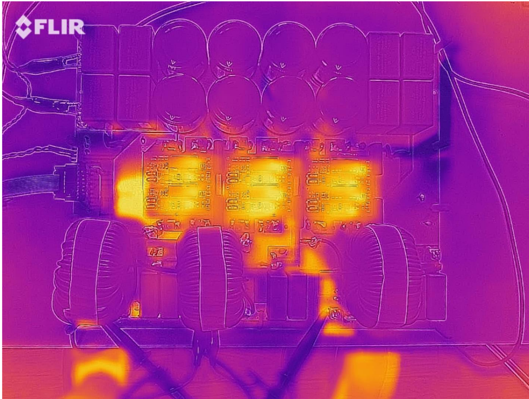
Figure 4.9. Photo for the circuit by using the Flir one pro thermal camera.
