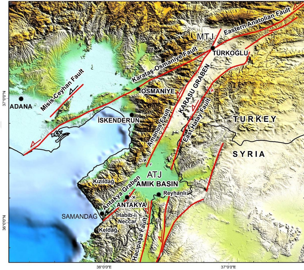
Figure 3.10. A digital elevation model for the study area and its surroundings, showing the major active faults and the morphotectonic units. MTJ: Kahramanmaraş or Türkoğlu Triple Junction, ATJ: Amik Triple Junction.
