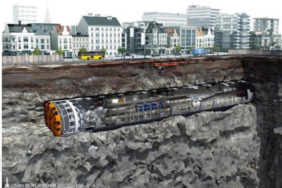
Figure 4.4 The advance of the TBM underground
