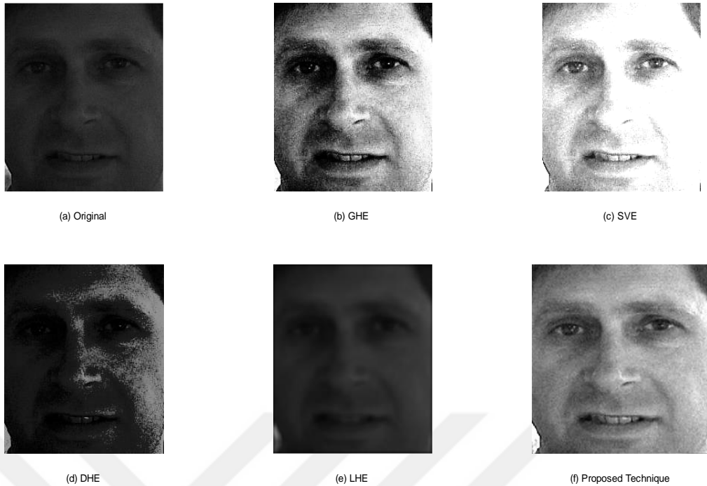
Figure 26. Low contrast face image from Caltech face database (a), Equalized image using: GHE (b), SVE (c), DHE (d), LHE (e), SVDWT image equalization technique (f)
