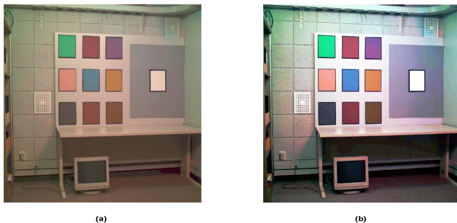
Figure 28. An image from [31] (a) and the equalized image using GHE in each R, G, and B channels separately (b).
