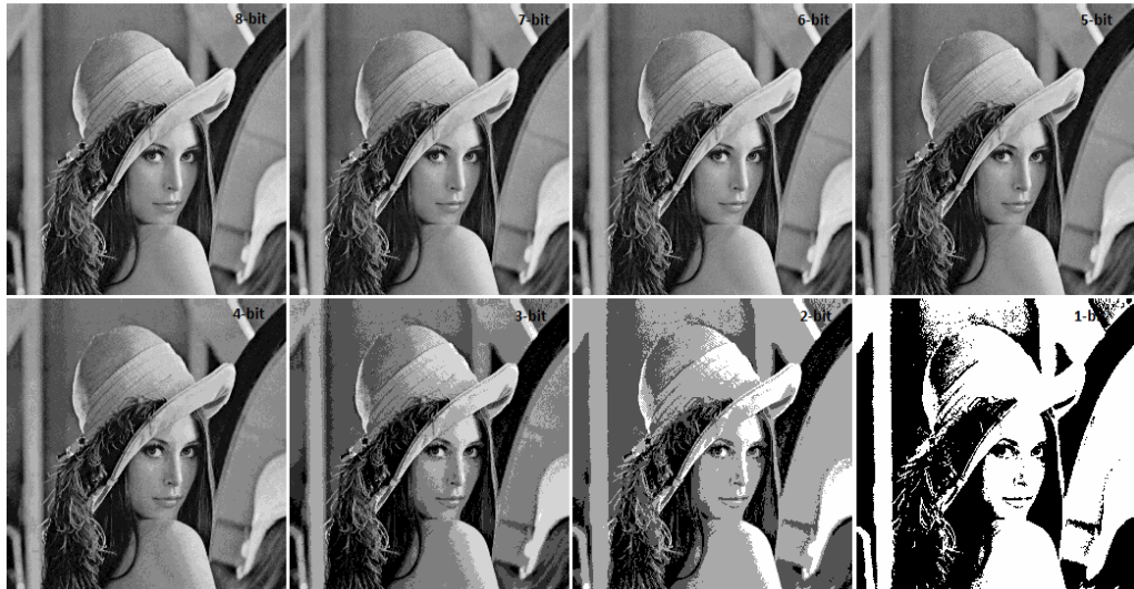
Figure 14. Gray Levels and Bit Depth of an Image
