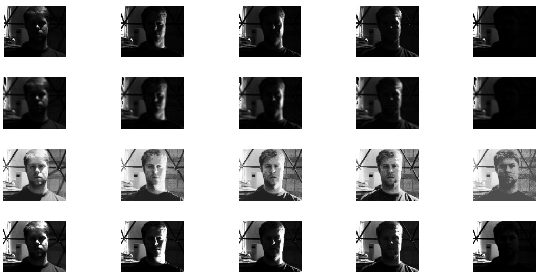
Figure 27. Low contrast faces images from Yale face database in the first row and the output of the LHE, GHE, and the SVDWT image equalization technique in the 2nd, 3rd, and 4th rows respectively.
