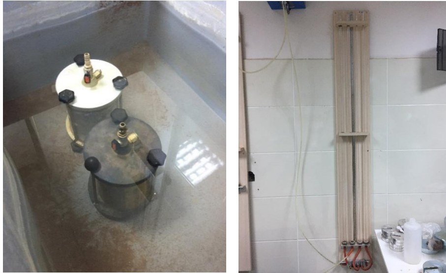
Figure 3.13 Falling head permeability test in laboratory.
