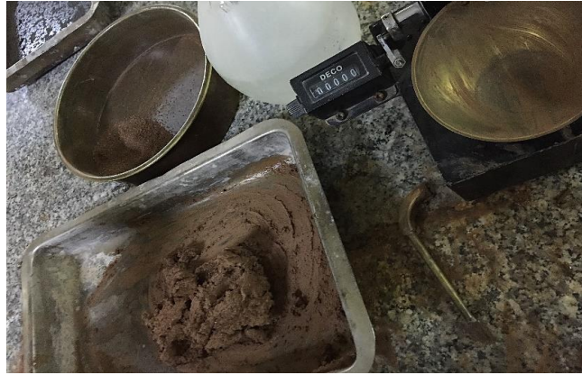
Figure 3.11 Determination of atterberg limits in laboratory.
