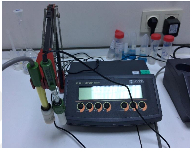
Figure 3.18 Conductivity and pH measurements.
