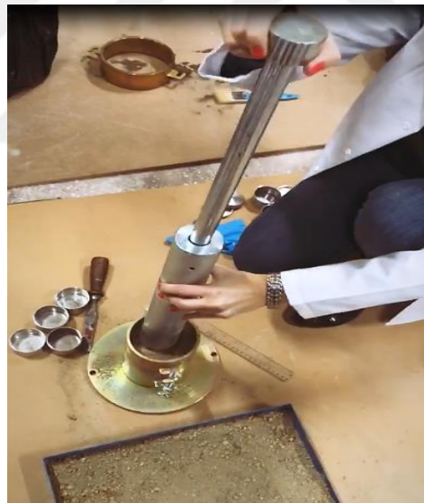
Figure 3.12 Standard compaction test in laboratory.
