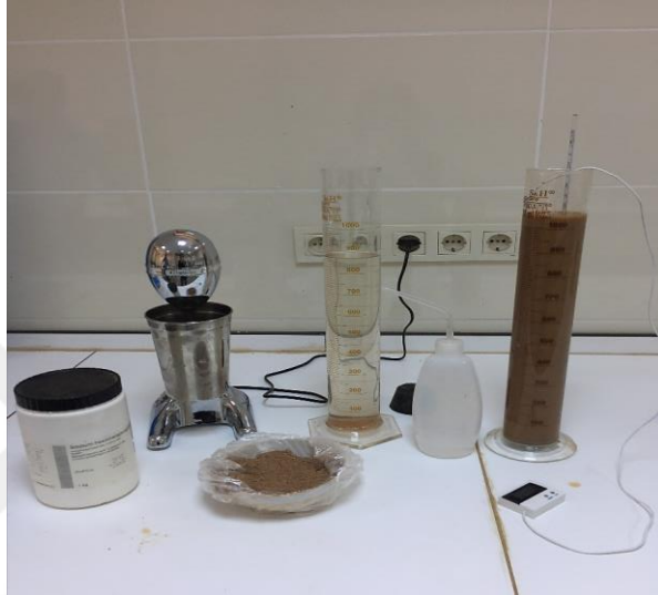
Figure 3.10 Hydrometer test in laboratory.
