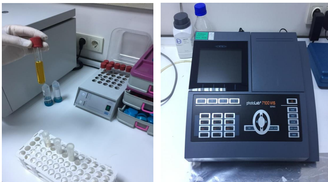
Figure 3.17 Disintegration sample in thermoreactor and spectrophotometer.
