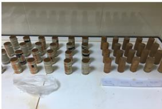
Figure 3.16 Photo of UCS specimens.
