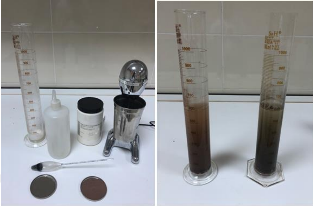
Figure 3.7 Hydrometer testing equipments' (left) and hydrometer testing on clay and sewage sludge ash (right)
