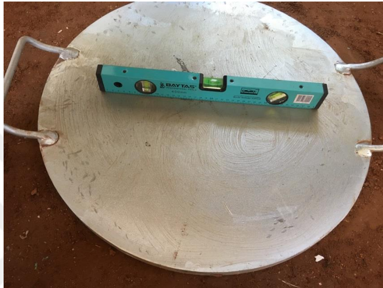
Figure 3.28 Photo of 30 cm diameter steel plate that used during the plate load test
