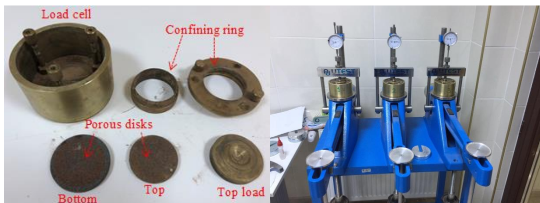
Figure 3.13 Photo of oedometer cell components and testing apparatus.
