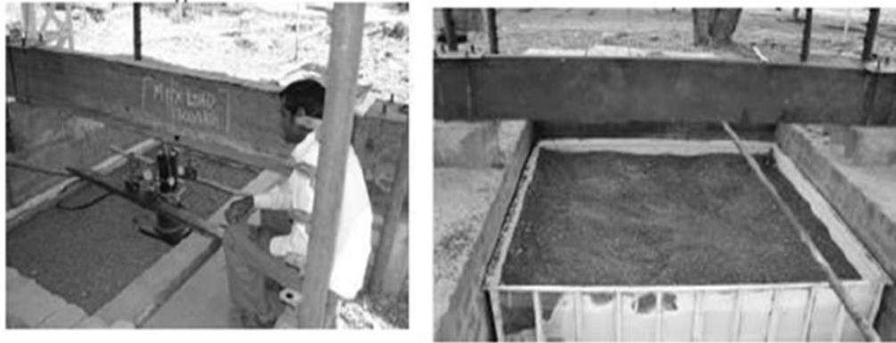
Figure 2.32 Image of the load test of the plate on the soil with granular layers (Sanjeev et al.,2013)
