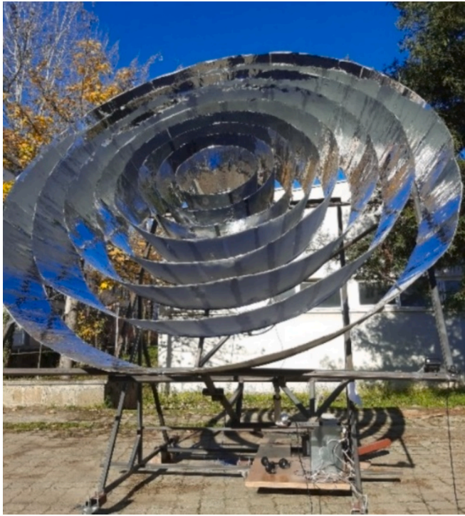
Fig. 4. Photo of eight-ring RAC system.
