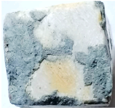
Type B failure mode on saw-cut surface
