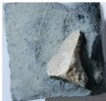
Type C failure mode on fractured surface
