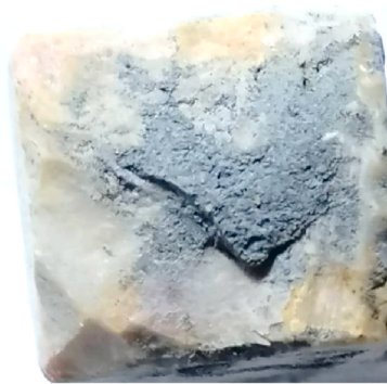
Type B failure mode on fractured surface
