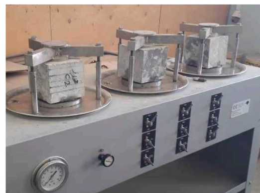
Fig. 5. Graphical representation and experimental set-up for permeability testing.
