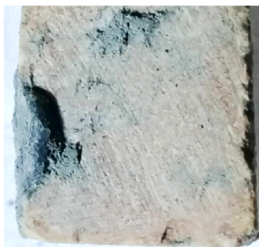
Type A failure mode on saw-cut surface
