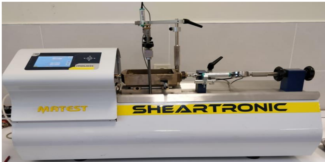
Figure 3.1 Schematic of the direct shear box
