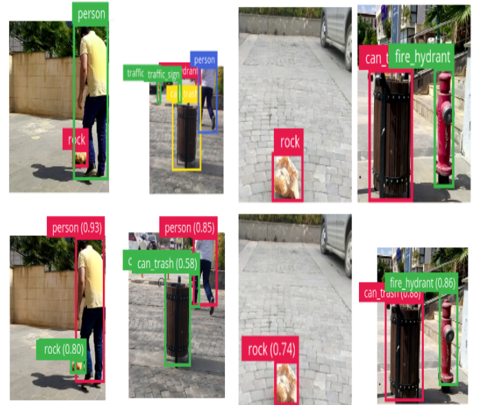
Fig 7: First row are the validation samples images with bounding boxes as ground truth and the second row are output from the object detection sub-system after fine-tuning with the pilot dataset with prediction confidence.
