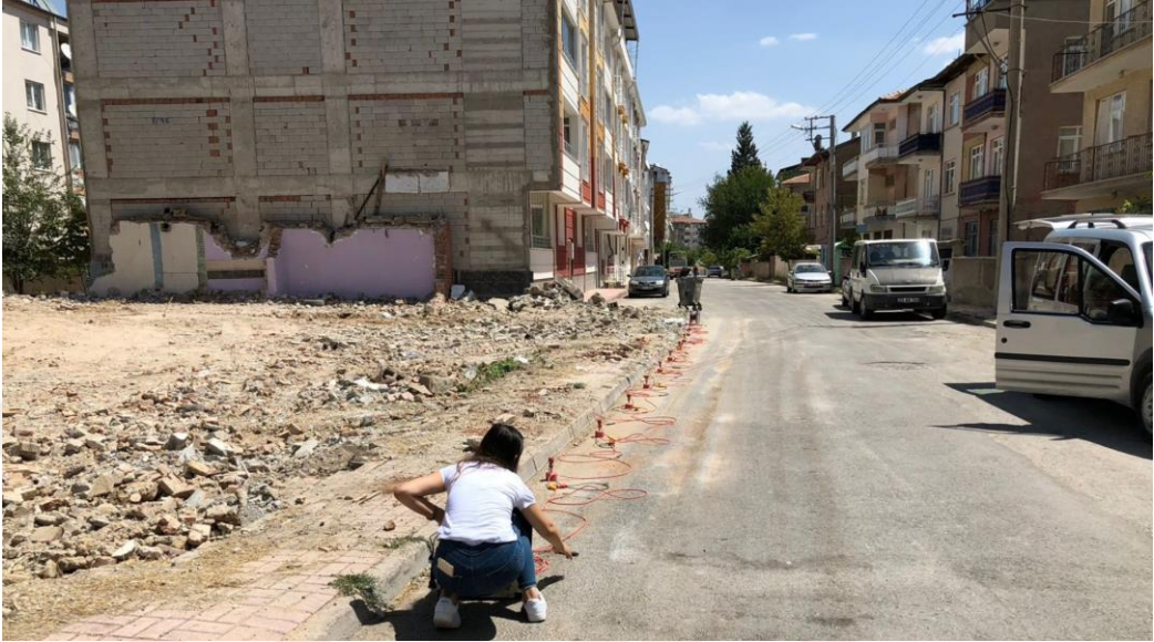
Figure 3.11. Application of MASW test in the field (photo)
