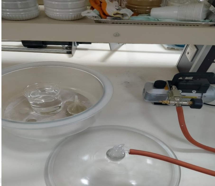
Figure 3.3. Photo of the elements used during the pycnometer test
