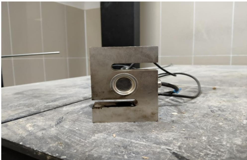
Figure 3.17. Photo of the S-type load cell
