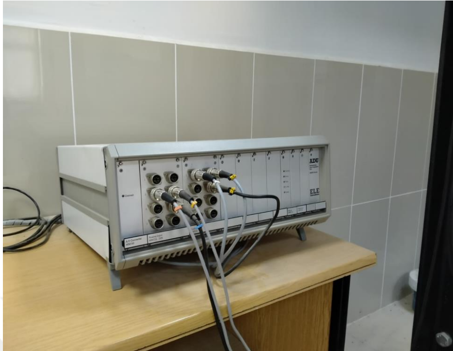
Figure 3.15. Photo of the data logger used during the tests
