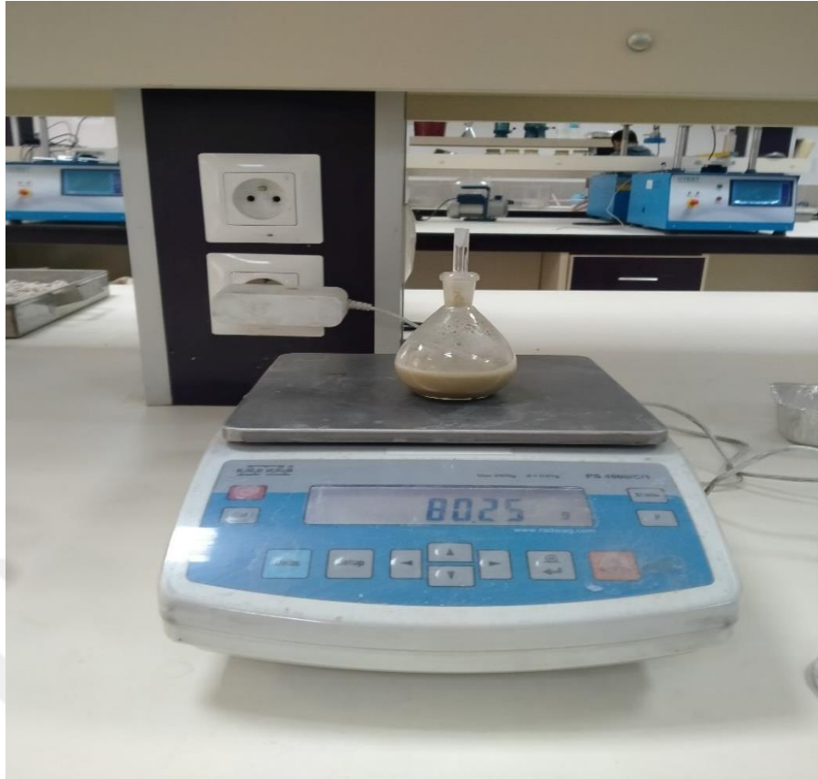
Figure 3.4. Photo of the weighing measurement during the pycnometer test
