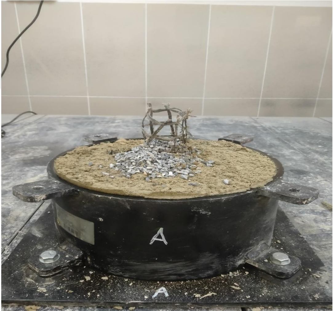
Figure 3.33. Photo of the plate loading test from the series 5
