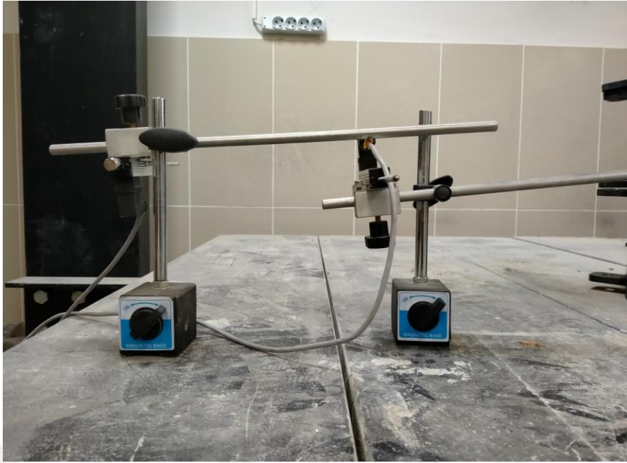
Figure 3.16. Photo of the displacement gauges
