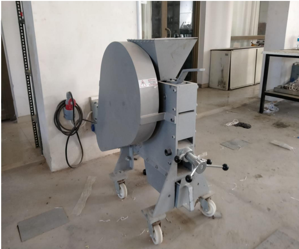
Figure 3.22. Photo of the grinding machine used to grind silt
