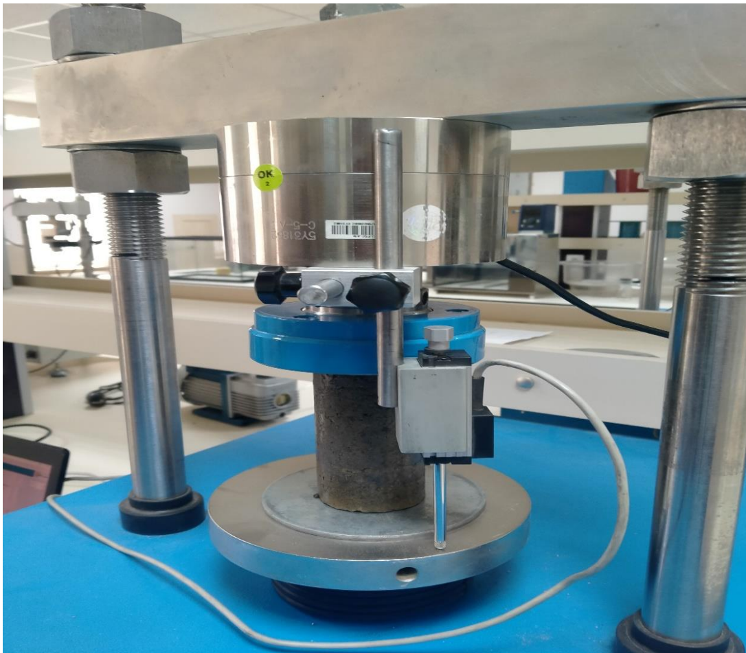
Figure 3.2. Photo of the unconfined compression equipment
