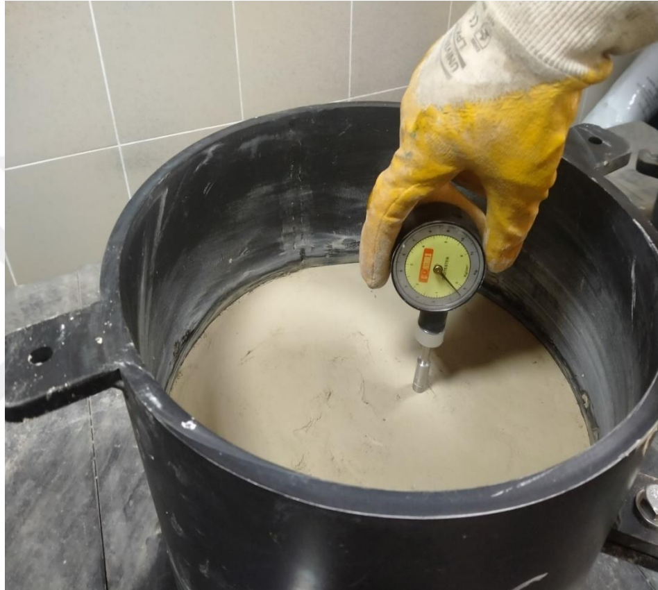
Figure 3.28. Photo of strength control of silty soil with a hand penetrometer
