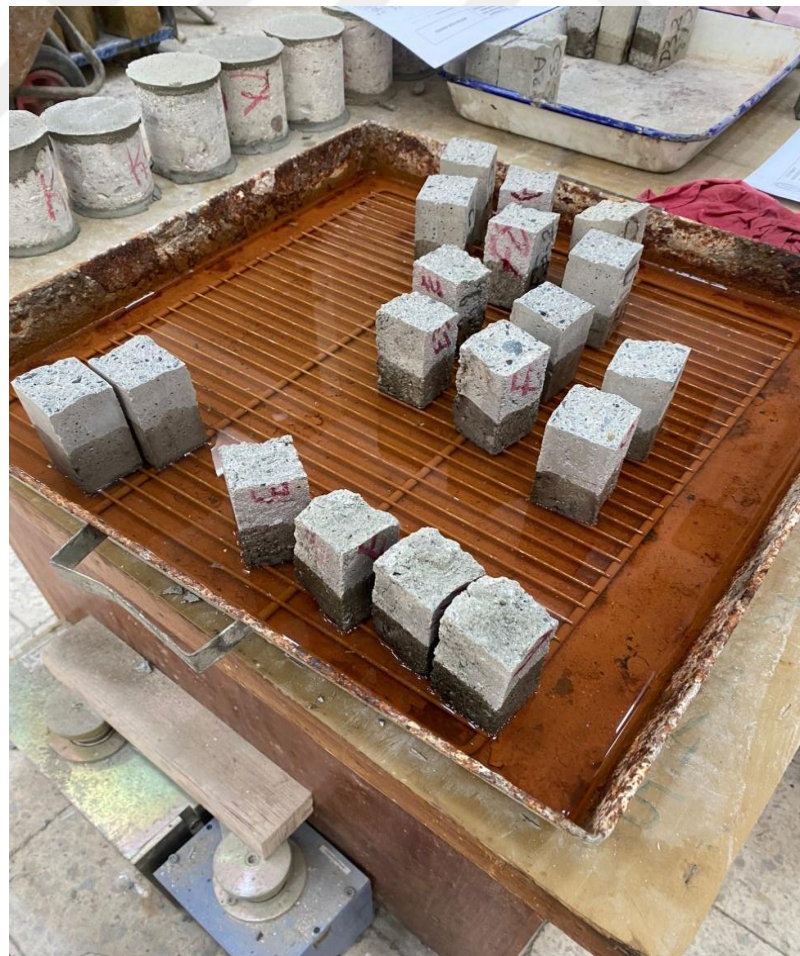
Figure 3.8: Capillary Water Absorption Test
