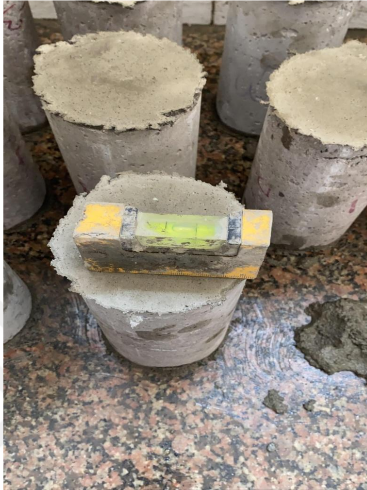
Figure 3.3: Cylinder Specimen Capping Process
