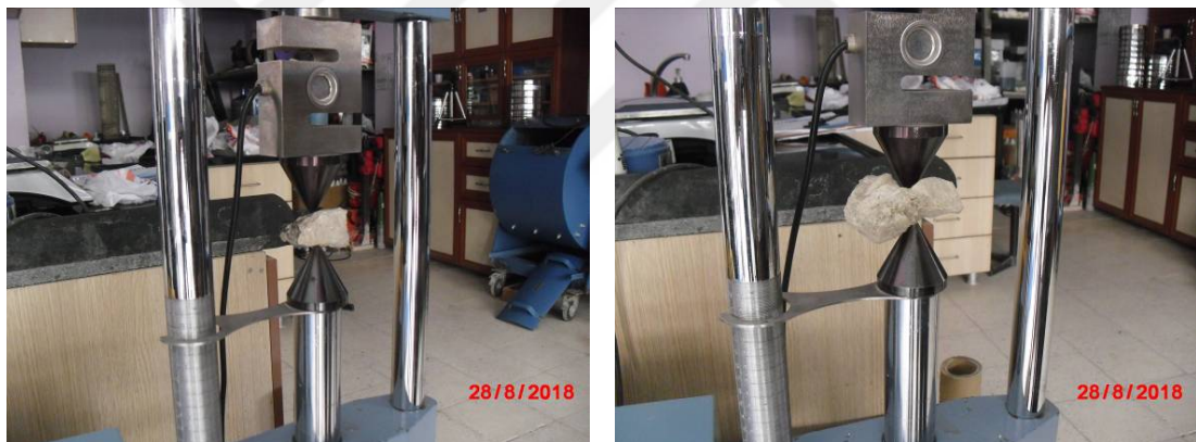
Figure 4.6: Point Load Test of Stone Samples
