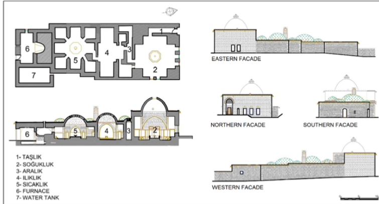
Figure 2. The architectural survey of the Eski Hamam. Plan, section, and elevations. (Source: Bebekoglu, 2005)
