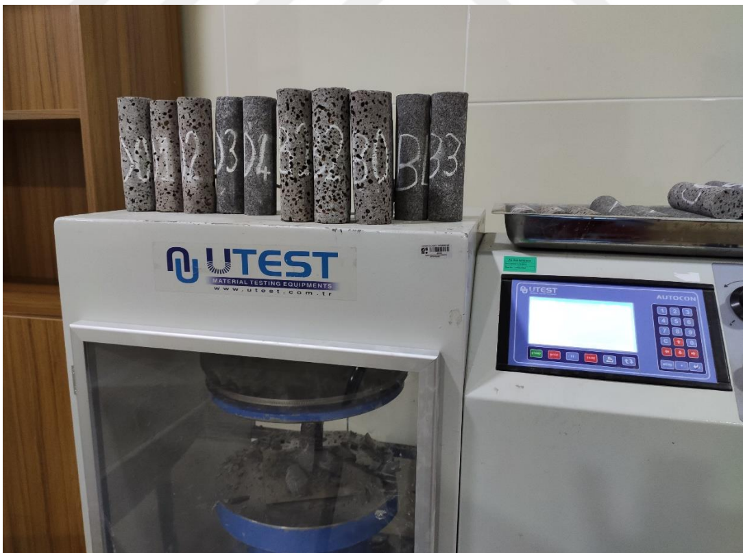
Figure 3.6. Uniaxial-compression testing device
