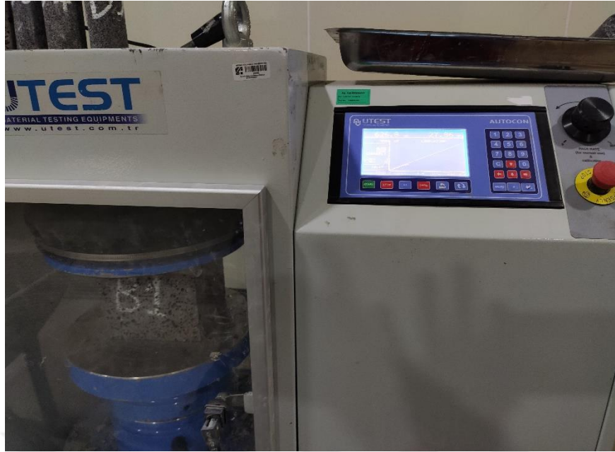
Figure 3.8. Infilled concrete sample Uniaxial compression test
