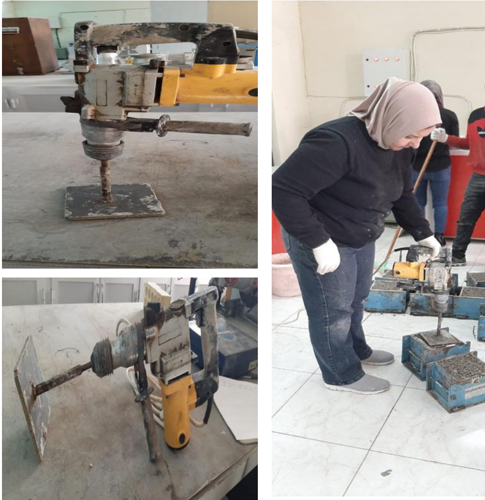
Figure 3.7 Compaction by jack hummer
