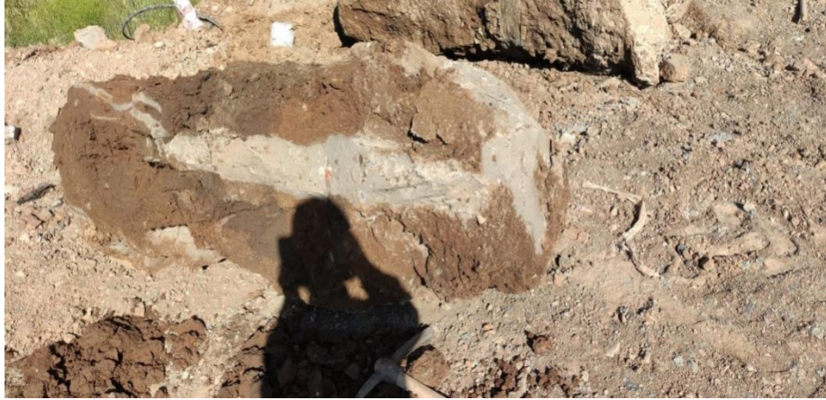
Figure 4.7 JG column manufactured with 300 bar
