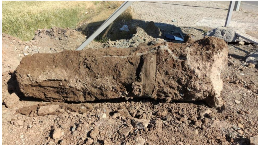
Figure 4.6 JG column manufactured with 450 bar
