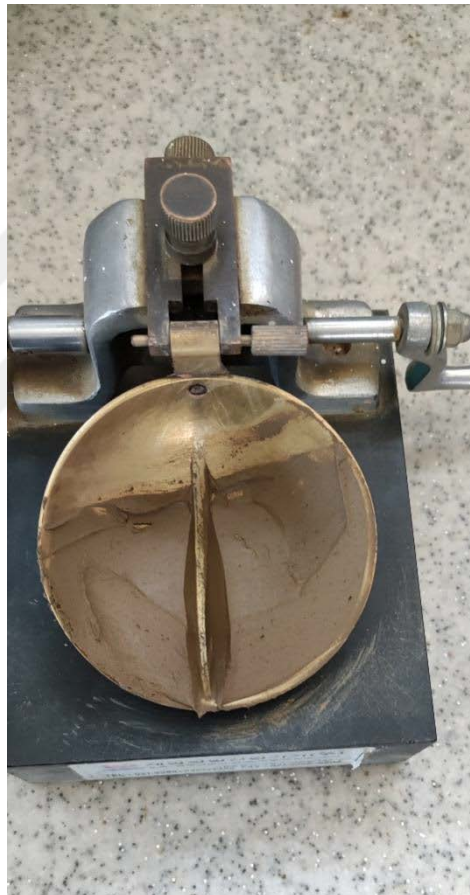
Figure 3.8 Liquid limit test
