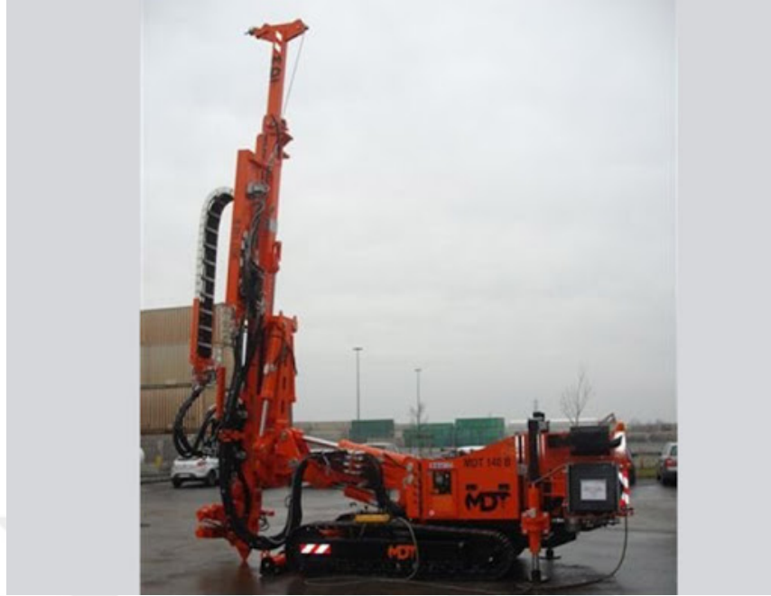
Figure 2.14 Punching machine for jet grout column
