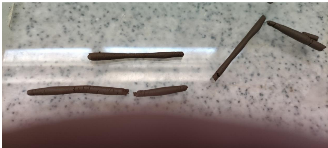
Figure 3.7 Plastic limit test
