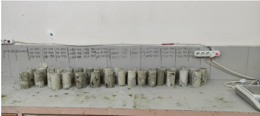
Figure 4.12 General appearance of samples subjected to free pressure experiment
