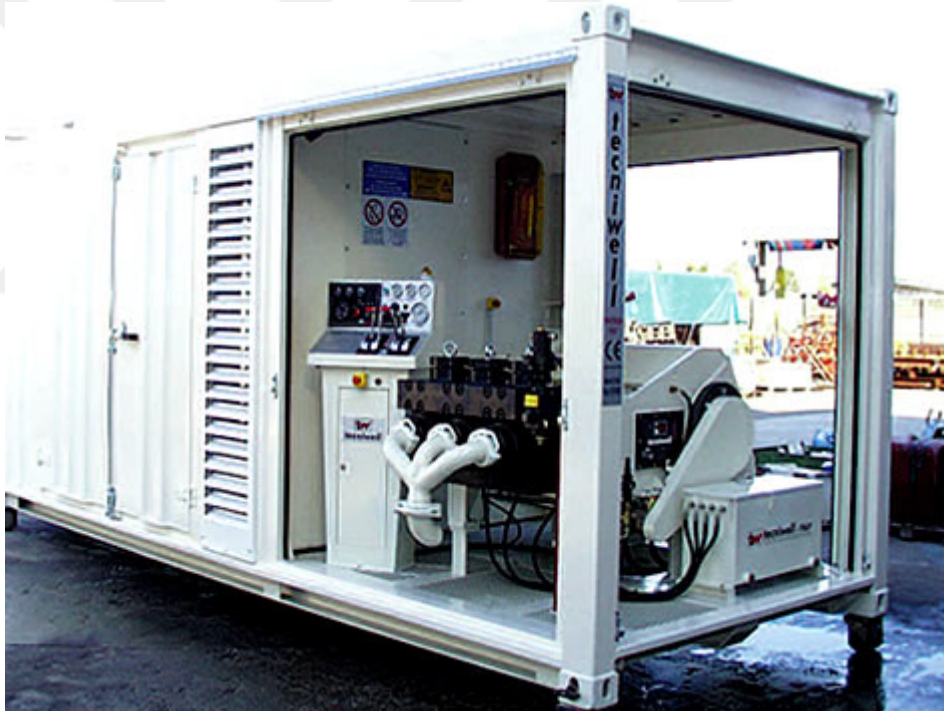
Figure 2.16 An image relating to the jet grout pump unit
