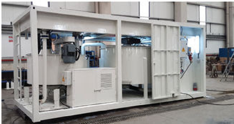
Figure 2.15 An image relating to jet Grout mixer unit.
