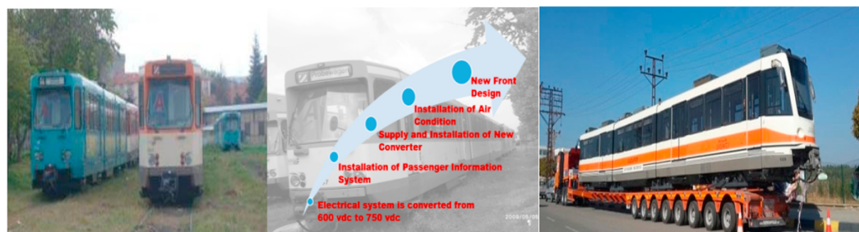
Fig. 4. Renovation of second-hand trams.
