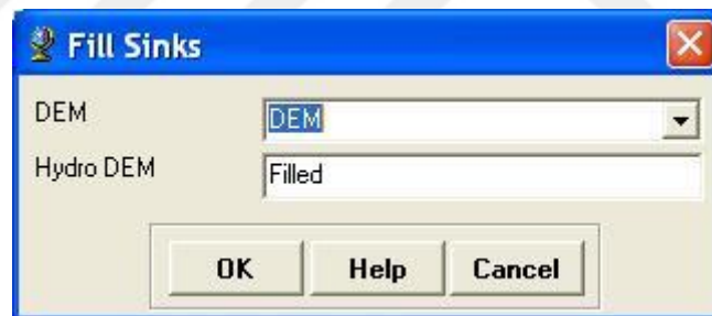
Figure 4.4 Filling sinks in ArcHydro
