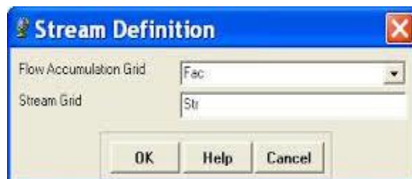
Figure 4.7 Stream definition step in ArcHydro
