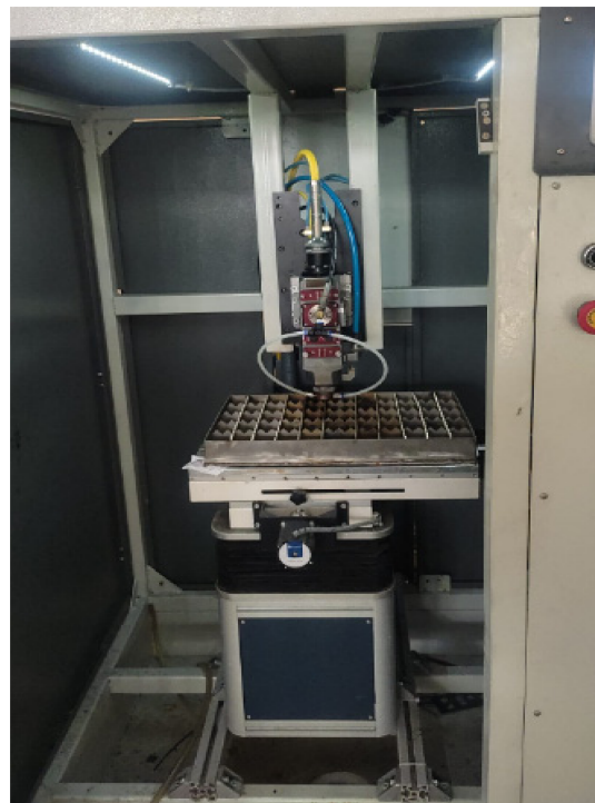
Figure 1. Design of waterjet-guided laser unit.
