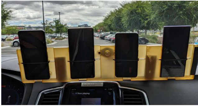
FIGURE 3. In-vehicle setup for gyroscope data collection using mounted smartphones [70], [74].
